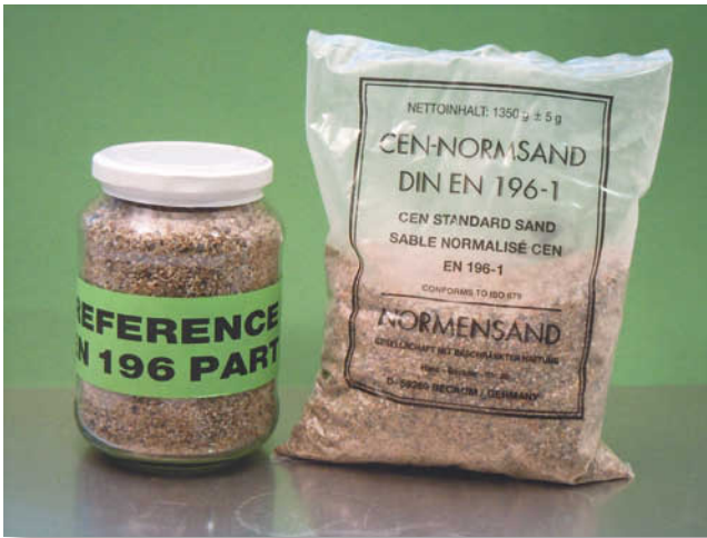
Figure 1: In accordance with EN 196-1, CEN standard sand must be packed in pouches containing 1350 ± 5 g. Three mortar prisms can be produced with one pouch. Specifying the pouch weight minimizes weighing errors in the laboratory. The CEN reference sand, i.e. the fundamental standard for the CEN test sand, is stored and sold in glass jars packed by Normensand GmbH.
